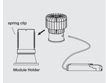
4. Attach module to module holder 5. Gently insert module holder with spring clip and connect module to driver.
